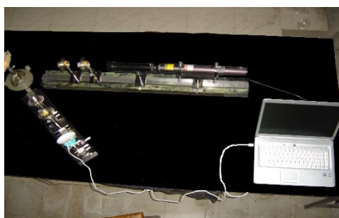
Figure1: Obtaining Mueller matrix elements: an experimental setup diagram
